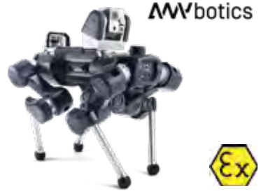
ROBOTIC INSPECTION - EX PROOF
