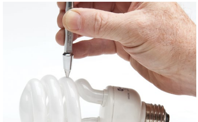
The High Resolution software option enables thickness measurements of up to 0.001 mm (0.0001 in.) resolution.
